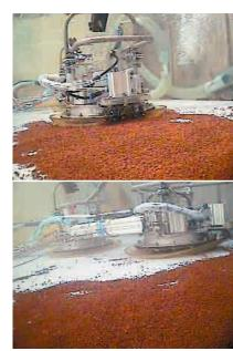
Suction-adheres to and freely moves along the surfaceof a wall, floor, etc. underwater <u>!!</u>
